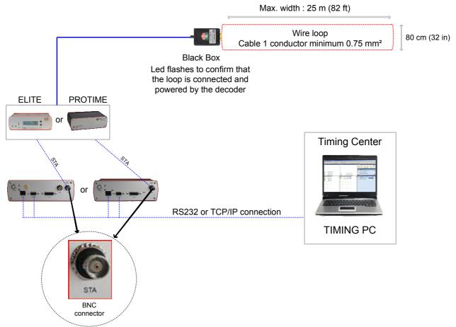
In some case, depending the speed, transponder position etc. you may set the loop width at 1 meter
