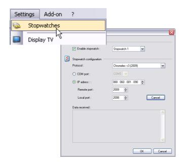
Firstly, you have to set the communication port of your computer. You may use a serial cable (with or without USB Adapter) or over Ethernet.
