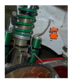
Wired Transponder as LS Wire or Elite Wire should be powered on +12V continuous power
