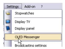
Enable the OLED Transmission on Elite and set the IP address of the computer were the Oled Messenger software is running. Remote port should be the same on OLED Messenger.exe
