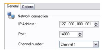
The Channel correspond to your setting in Elite v3. Different display settings can be set on each channel.
