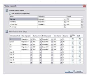
If you set a distance, Elite will automatically consider it as a speed measuring zone and calculate the average speed. The "speetrap" should always have more than 10 meters for speeds over 100km/h (60mph) in order to get a reliable measure.
